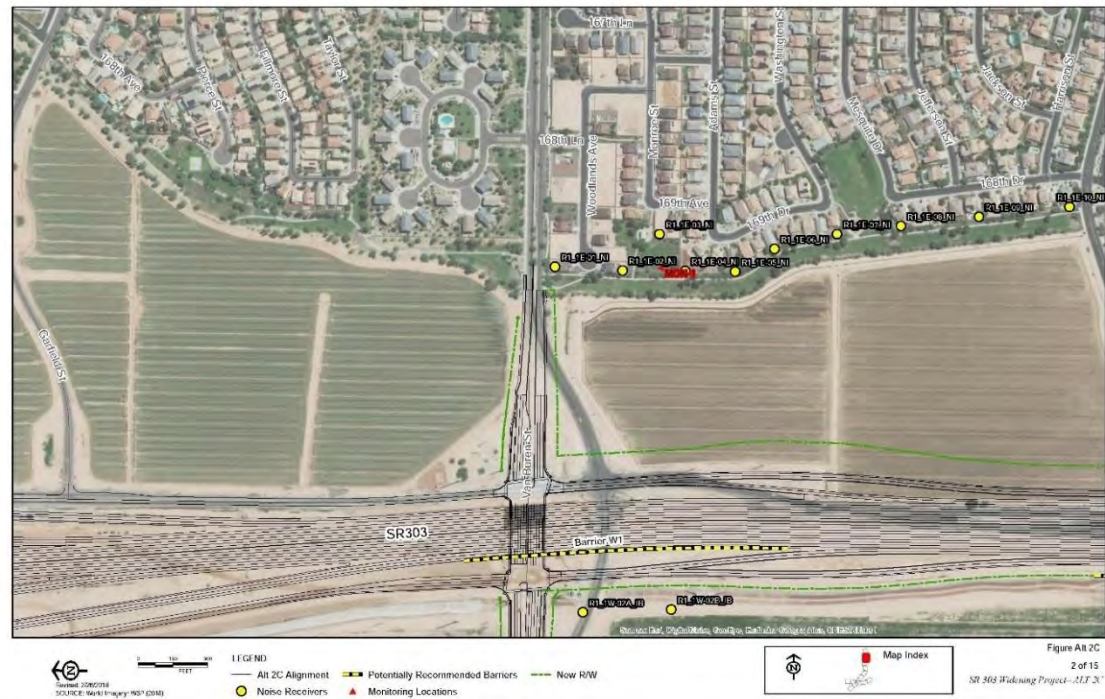
Figure 5-16: General Noise Wall Requirements
