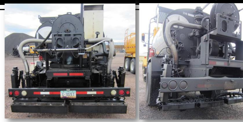
Each truck was used the same amount of time; one with "Spray Guard" the other without. Notice the break/reverse lights and reflective tape.
