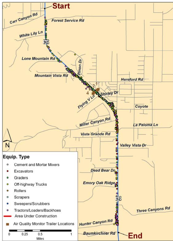
Figure 8-35. Construction activity locations, April 13-17, 2009 (workdays during the case study week of April 13-19; based on GPS tracking reported every five minutes).
