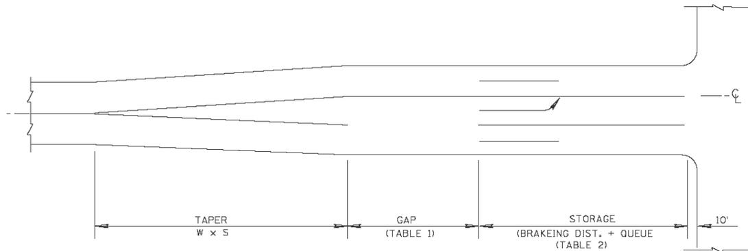
The preferred way of creating a left turn lane is by widening the roadway on both sides equally as shown in Figure 430-B. This minimizes the amount of lateral shifting required for through traffic.
