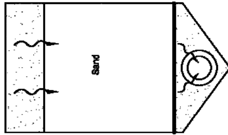
Sand Filter with Gravel Pretreatment
