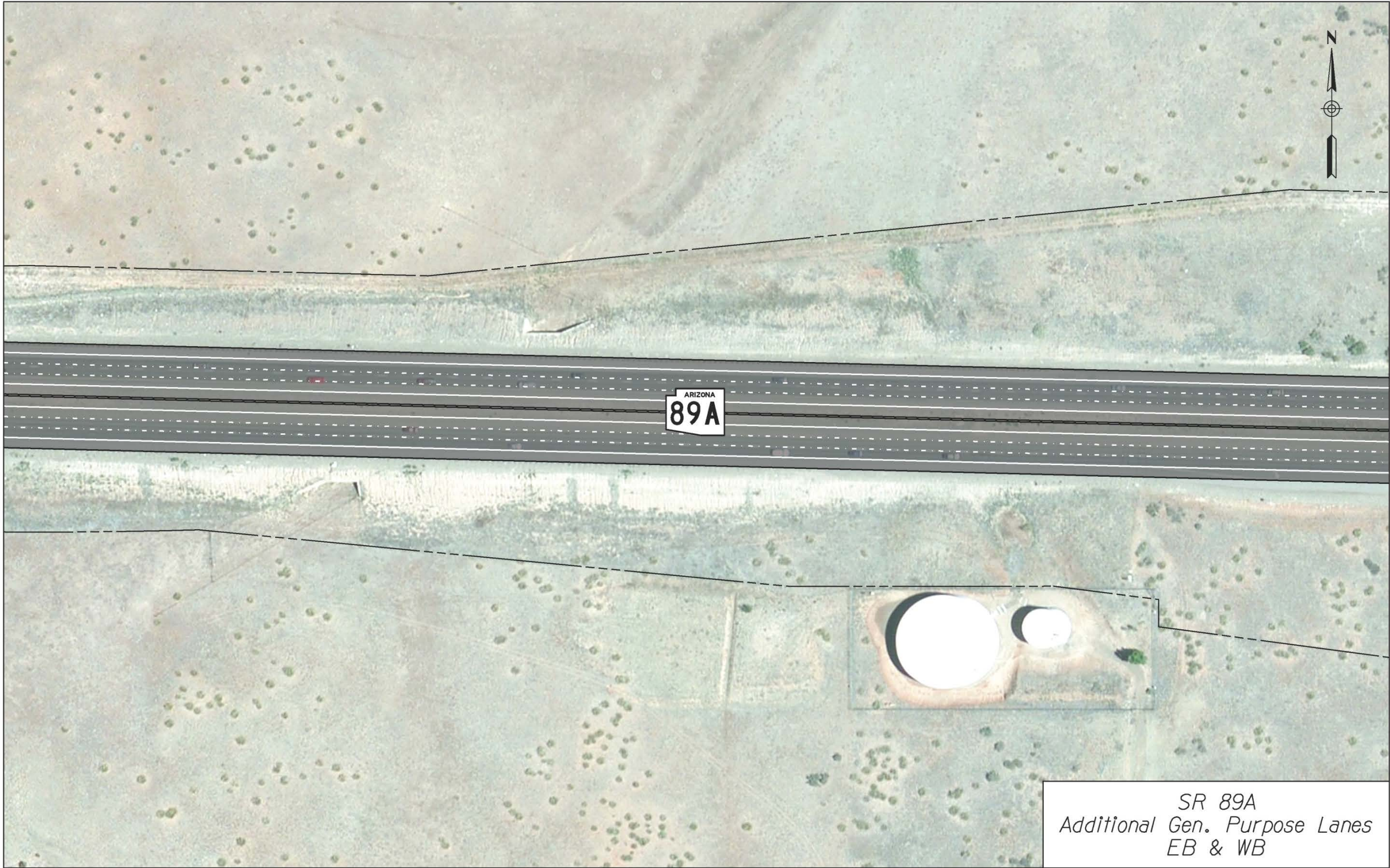
Figure 27: General Purpose Lane Widening
