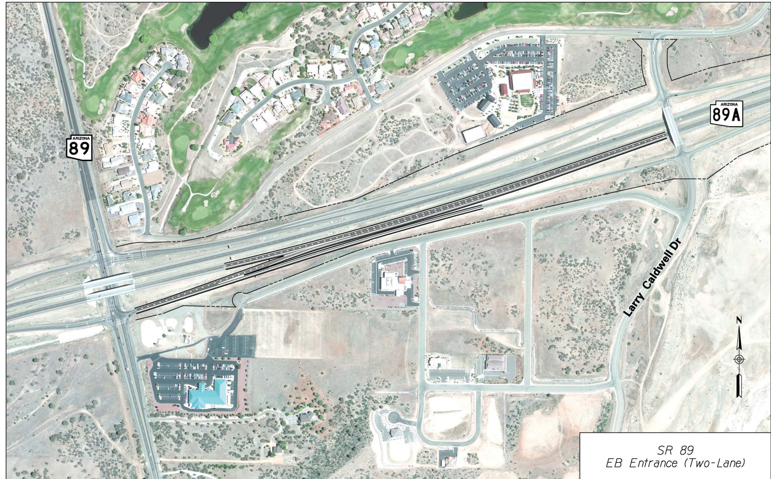
Figure 30: SR 89 TI Eastbound Entrance Ramp Option 2
