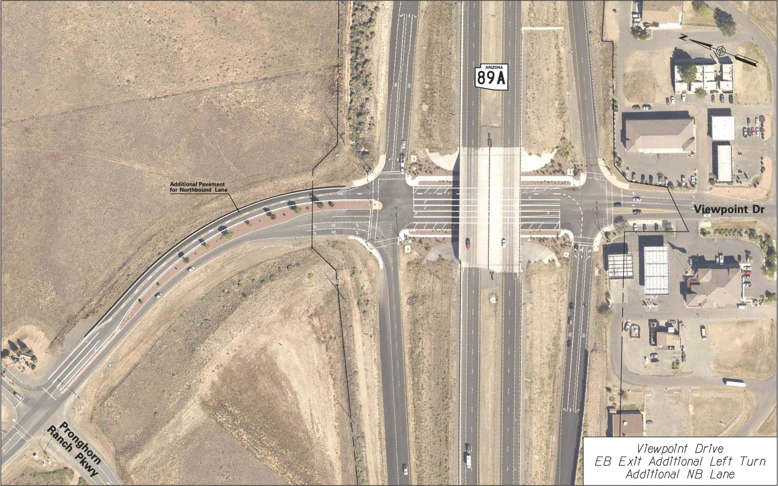
Figure 38: Viewpoint Drive TI Additional Northbound Lane and Eastbound Dual Left-Turn
