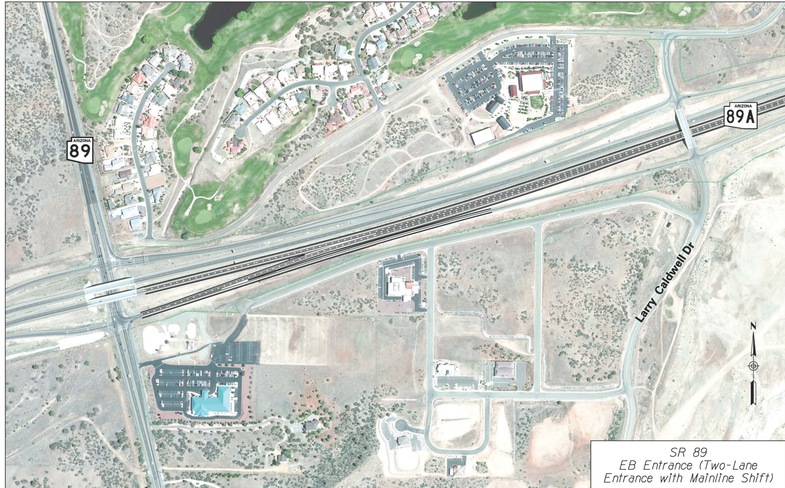
Figure 29: SR 89 TI Eastbound Entrance Ramp Option 1
