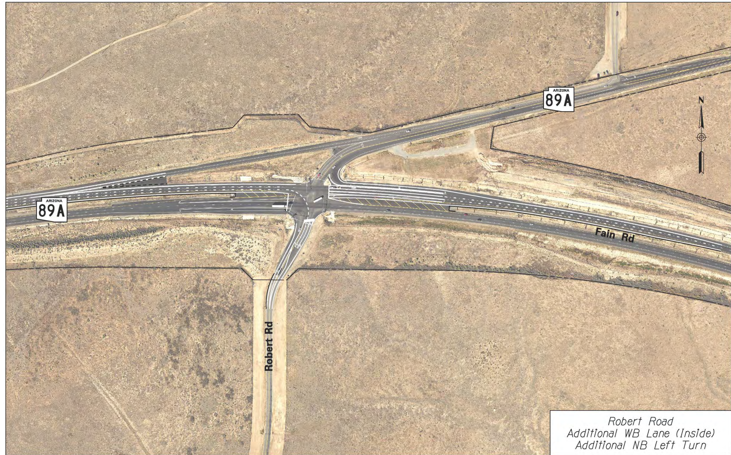
Figure 41: Robert Road Signalized Intersection Improvements
