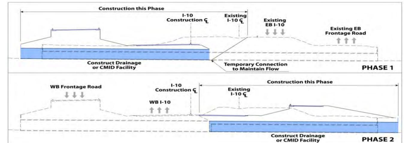
Figure 4.7 – Proposed Drainage/Utility Facility Construction
