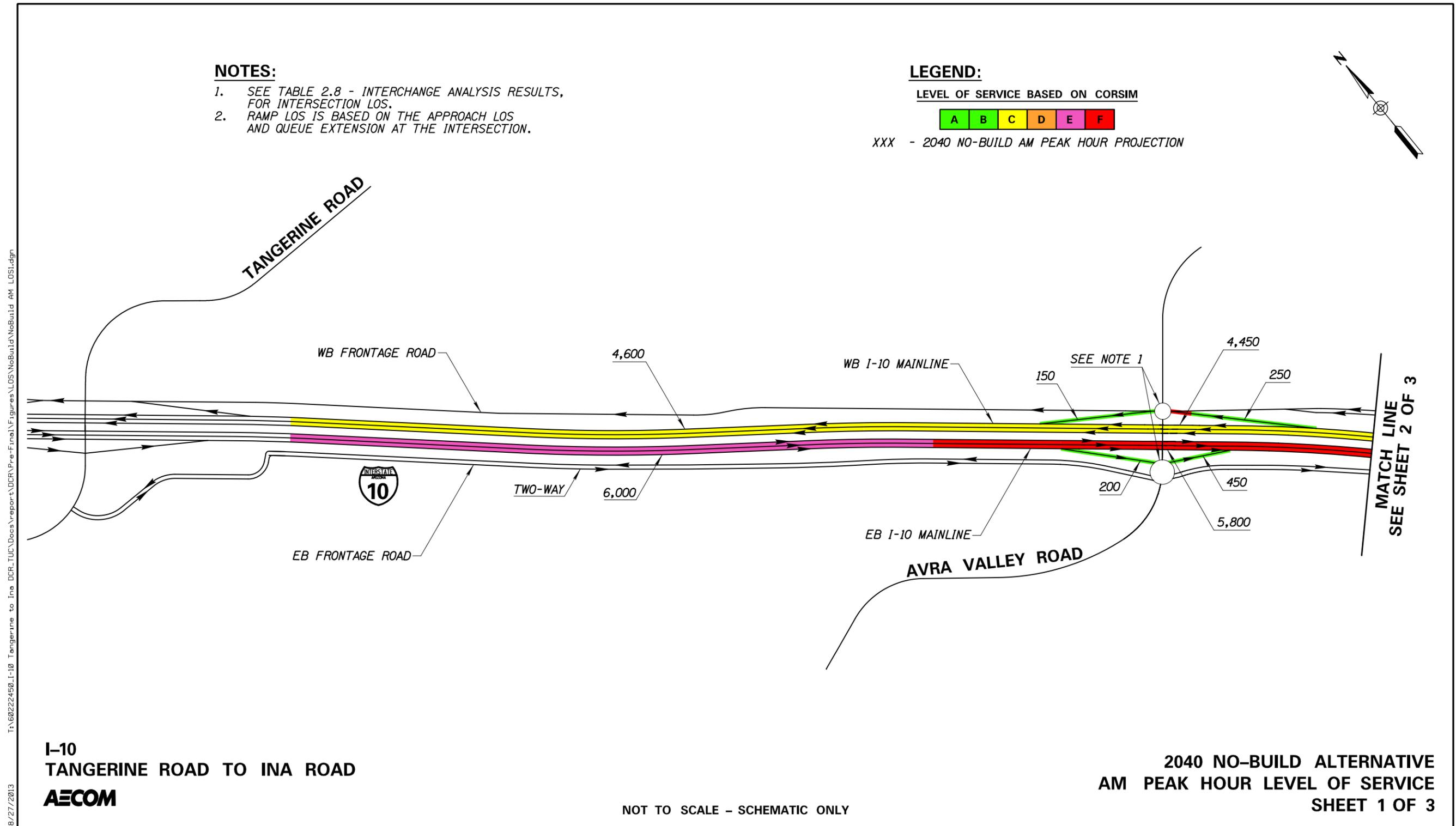
Figure 2.7 – 2040 No-Build Alternative AM Peak Hour Level Of Service
