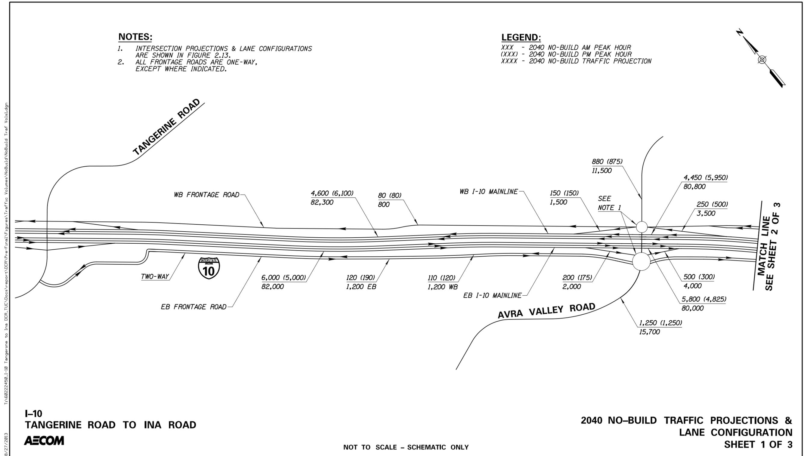
Figure 2.3 – 2040 No-Build Traffic Projections & Lane Configuration
