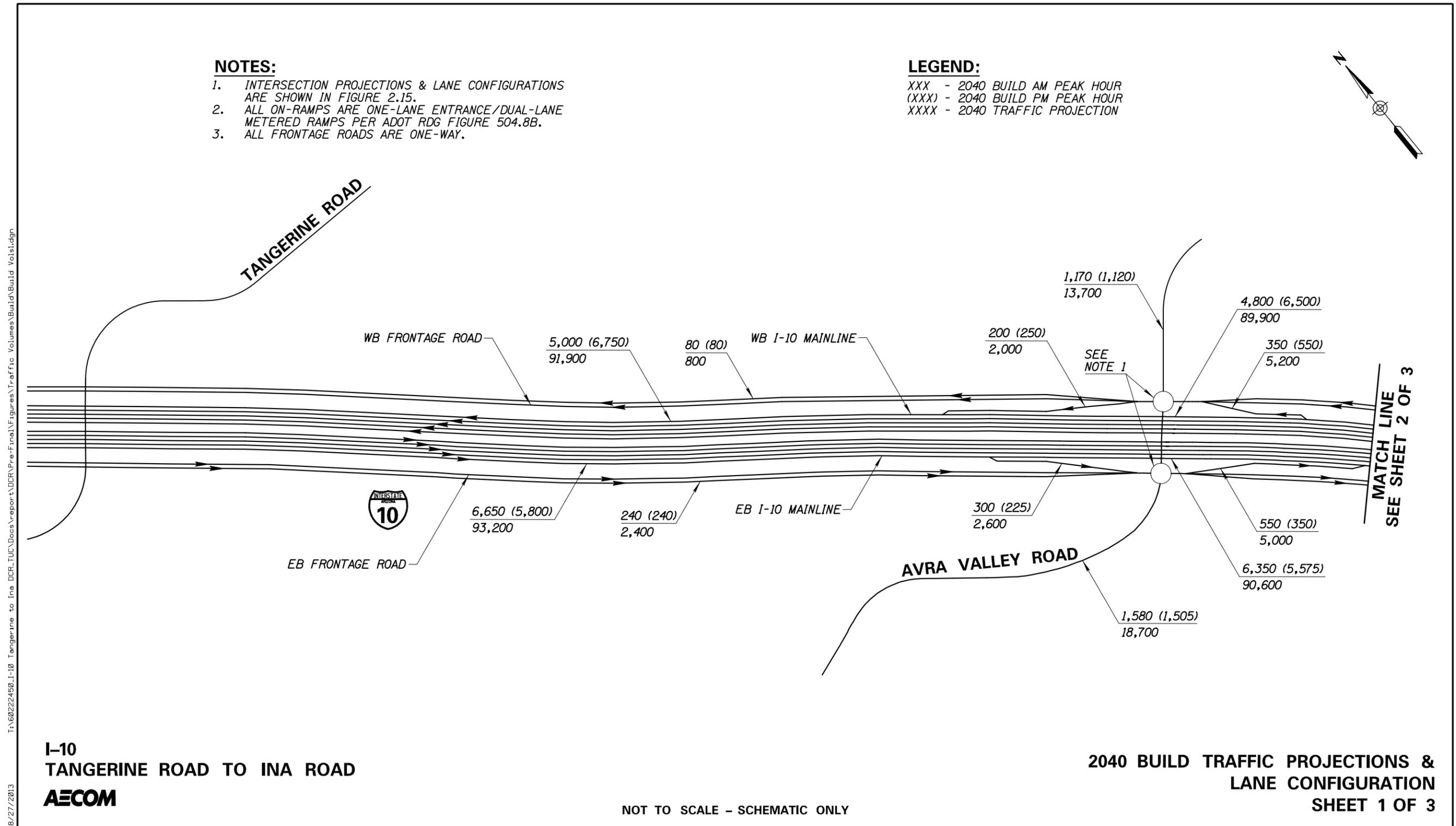
Figure 2.4 – 2040 Build Traffic Projections & Lane Configuration
