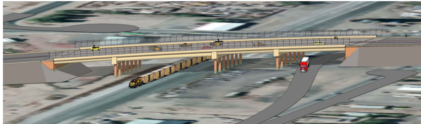
Figure 4-6: 3D Rendering of Recommended Bridge Structure
