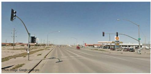
What appears to have been crosswalk stripping between the west side of US-191 and the sidewalk at the southeast corner of the intersection is all but obliterated (Figure 2.12). Similarly, extremely faded crosswalk stripping is present for the crossing between the southeast and northeast corners of this intersection (Figure 2.13).
