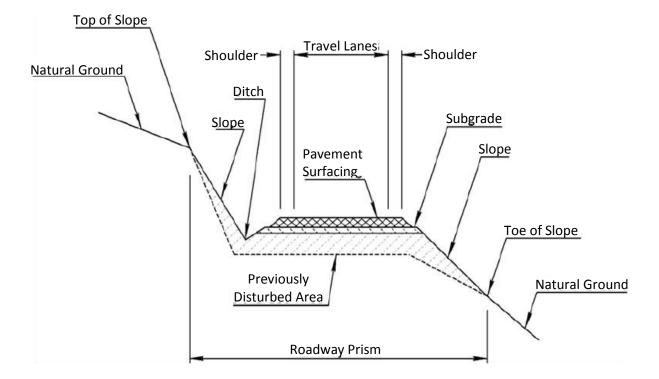
Figure 1. Illustration of Roadway Prism
