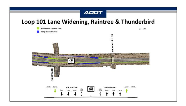
As we move further south along the project. The existing freeway transitions from an elevated freeway near Frank Lloyd Wright to a depressed condition near Raintree. The existing bridges over Loop 101 at Raintree Drive and Thunderbird Road have adequate length and will not need modifications to make room for the additional general purpose lane.
