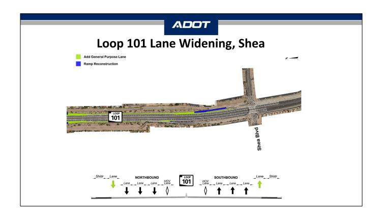
This slide shows the southern limits of the project, where the project improvements tie into the previously completed project that added a general purpose lane along Loop 101 from Shea Blvd to the Loop 202 Red Mountain Freeway. I would like to note that the project design minimizes the improvements to the southbound Shea Blvd Exit Ramp to avoid impacts to the existing aesthetics located on the existing walls.
