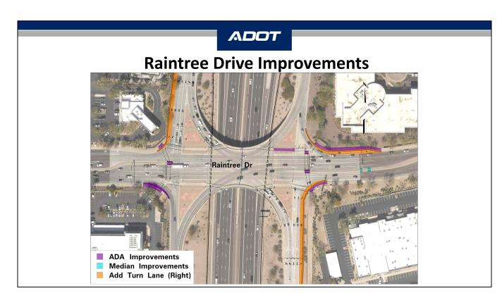
At Raintree Drive the majority of the interchange will remain as it is today. However, right turn bays will be added for the NB to EB, WB to NB, and SB to WB movements.
