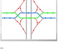
The second option is a Diverging Diamond Interchange (DDI) with signalized ramps to and from I-10.
