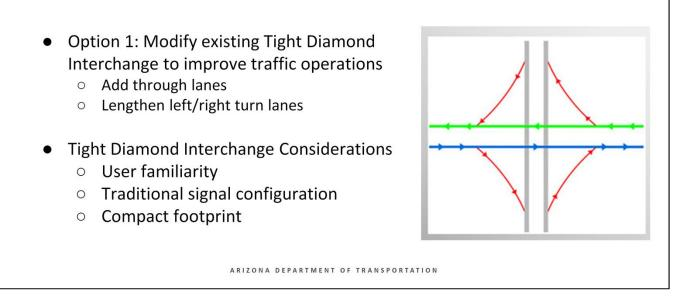
The first option for improving the traffic interchange that was recommended for advancement in the feasibility study was for the interchange to remain a tight diamond, with features intended to improve operation of the interchange and reduce vehicle queues.
