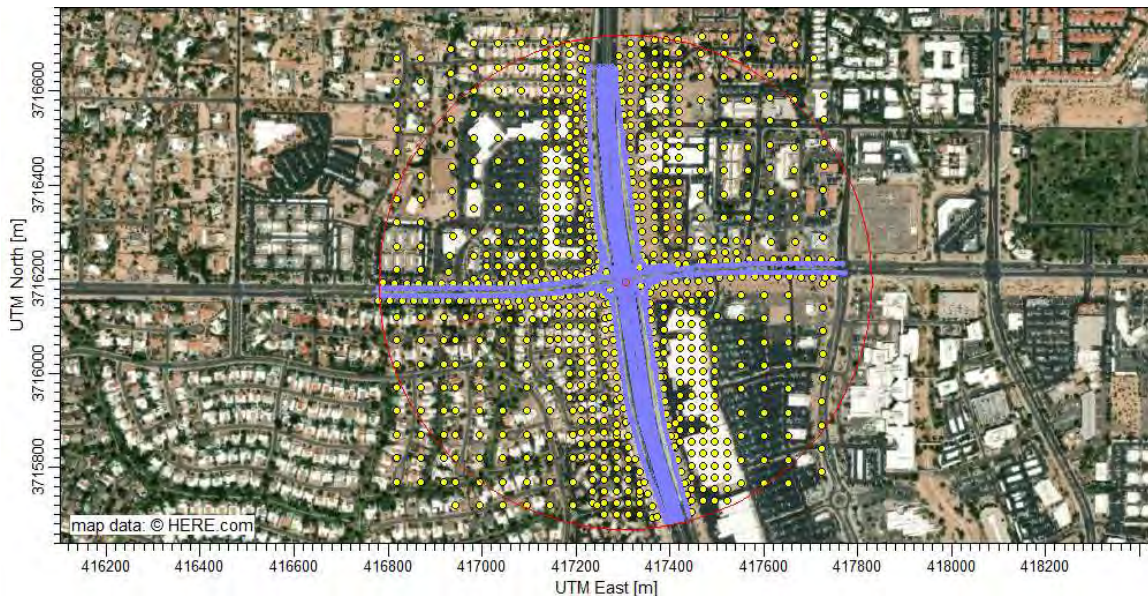
Figure 17. SR101 and Shea Boulevard PM 10 Receptor Locations
