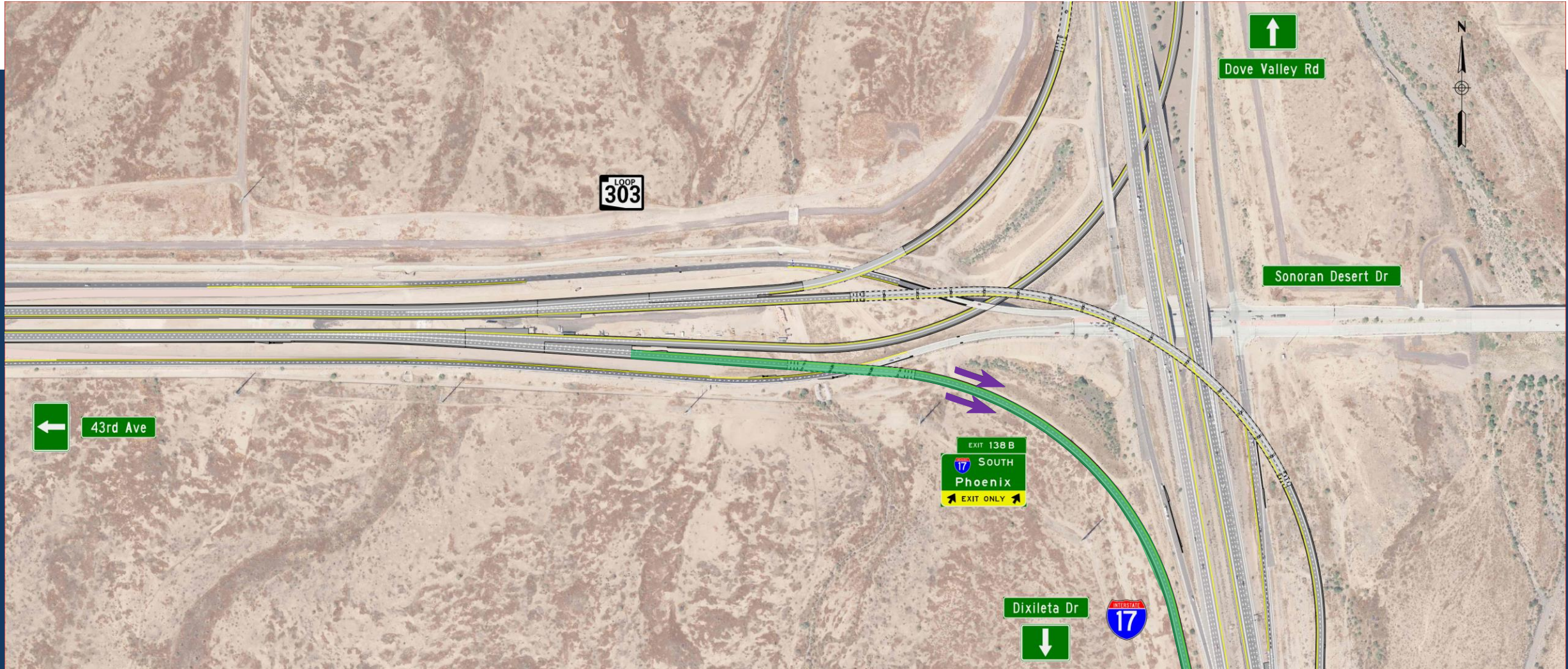
L303 to SB I-17 Direct Access Ramp
