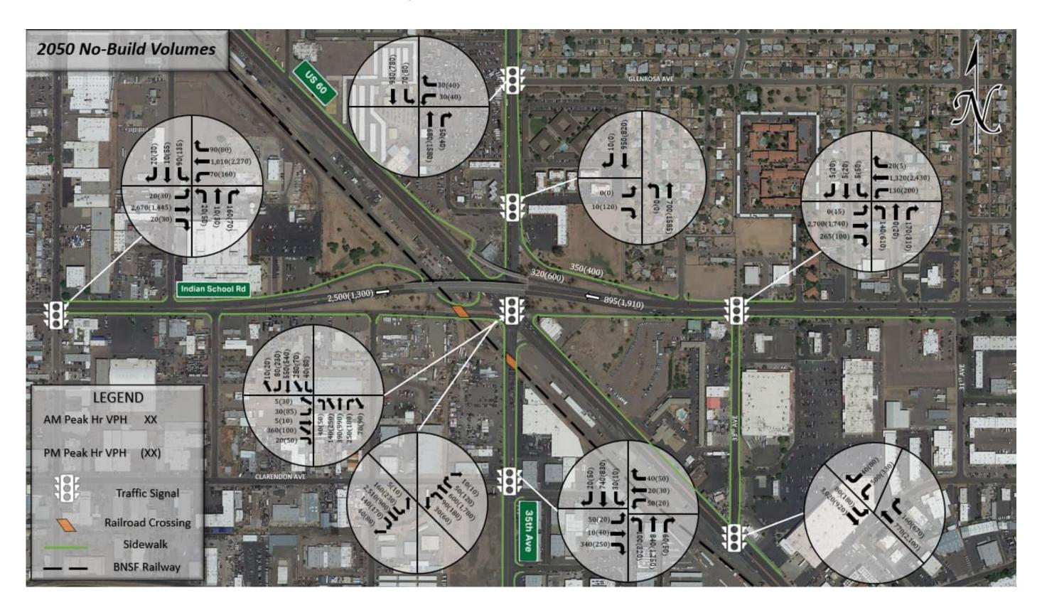
Figure 13 – 2050 No-Build Conditions Lane Configurations
