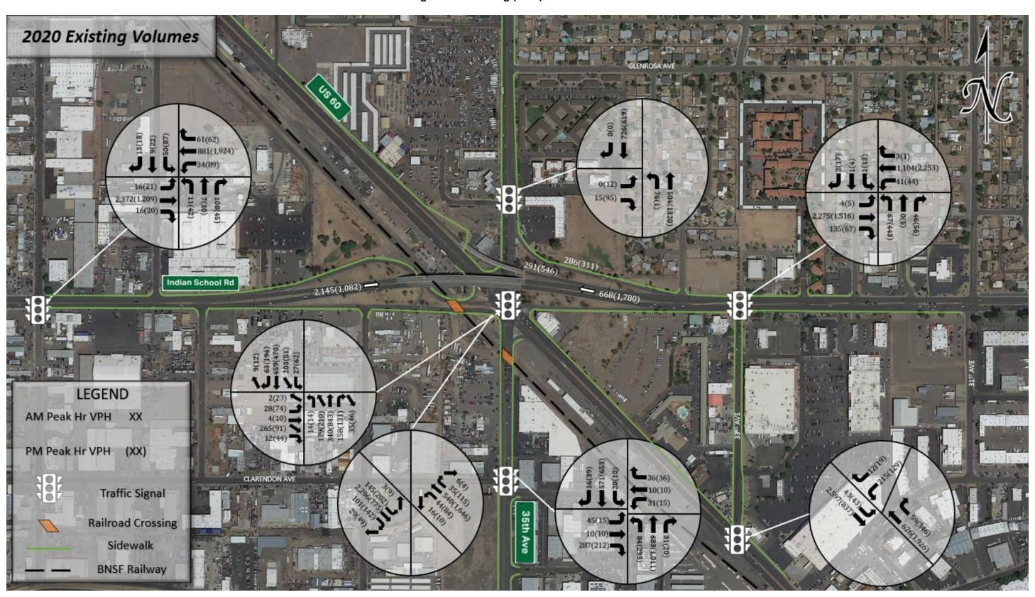
Figure 11 – Existing Lane Configurations
