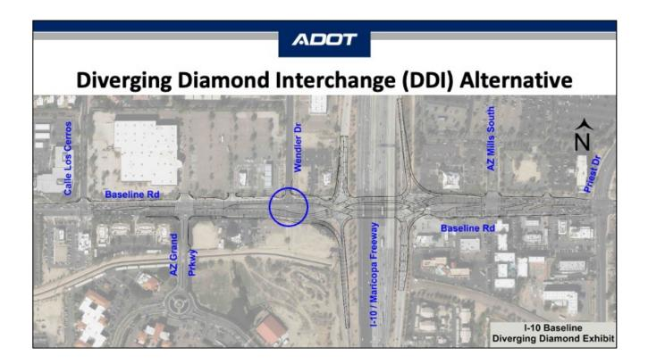
This alternative also includes the removal of the traffic signal at Wendler Drive and revises Wendler access to be right-in, right-out. This will improve the flow of traffic on Baseline Road by reducing conflict points and extending the available queue area approaching I-10.
