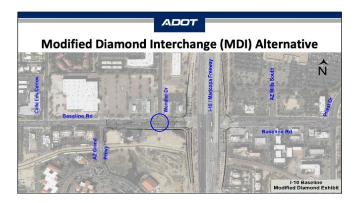
This alternative also includes the removal of the traffic signal at Wendler Drive and revises the access to be right-in, right-out. This will improve the flow of traffic on Baseline Road by reducing conflict points and extending the available queue area approaching I-10.
