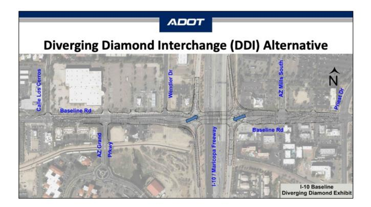
Again, the DDI would increase traffic flow by traffic temporarily transitioning to the left side of the road, allowing through-traffic and left-turning traffic to proceed through the interchange simultaneously, eliminating the need for a signalized left-turn. DDIs are particularly effective at locations that have high volumes of left-turn traffic on and off of freeway ramps and left-turn related safety challenges.
