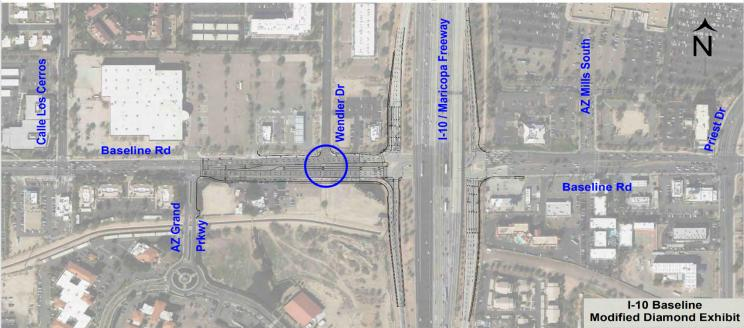
This alternative also includes the removal of the traffic signal at Wendler Drive and revises the access to be right-in, right-out. This will improve the flow of traffic on Baseline Road by reducing conflict points and extending the available queue area approaching I-10.
