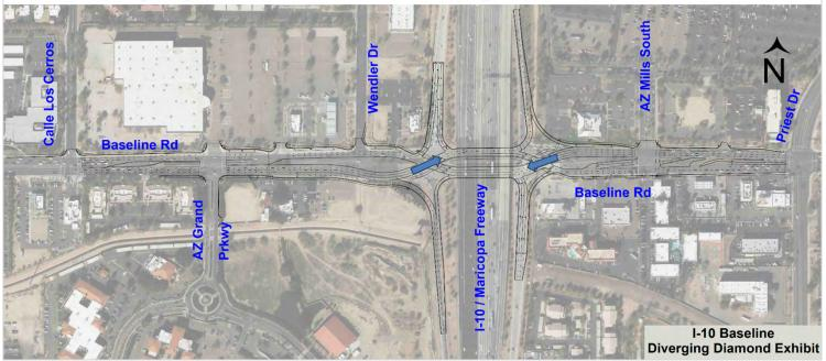
Again, the DDI would increase traffic flow by traffic temporarily transitioning to the left side of the road, allowing through-traffic and left-turning traffic to proceed through the interchange simultaneously, eliminating the need for a signalized left-turn. DDIs are particularly effective at locations that have high volumes of left-turn traffic on and off of freeway ramps and left-turn related safety challenges.
