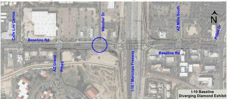
This alternative also includes the removal of the traffic signal at Wendler Drive and revises Wendler access to be right-in, right-out. This will improve the flow of traffic on Baseline Road by reducing conflict points and extending the available queue area approaching I-10.
