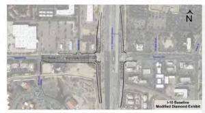
The Modified Diamond alternative would keep the interchange and ramp configuration as they are while adding some modifications to improve traffic operations, including adding new right turn lanes on Baseline Road at I-10 and additional lanes on the exit and entrance ramps. This alternative includes the removal of the traffic signal at Wendler Drive and revising access to be right-in, right-out.
