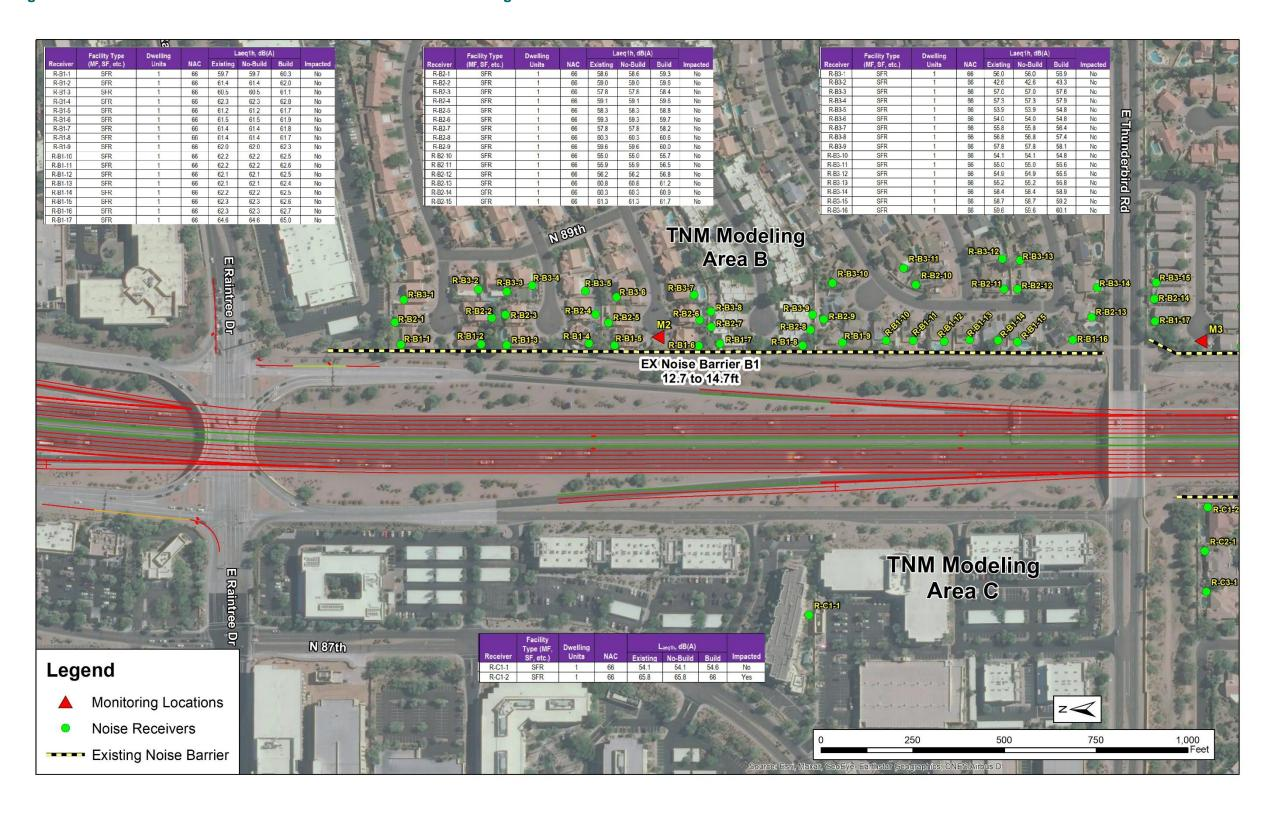
Figure 13. E Thunderbird Rd. to E Sweetwater Ave. – Receiver and Existing Barrier Locations
