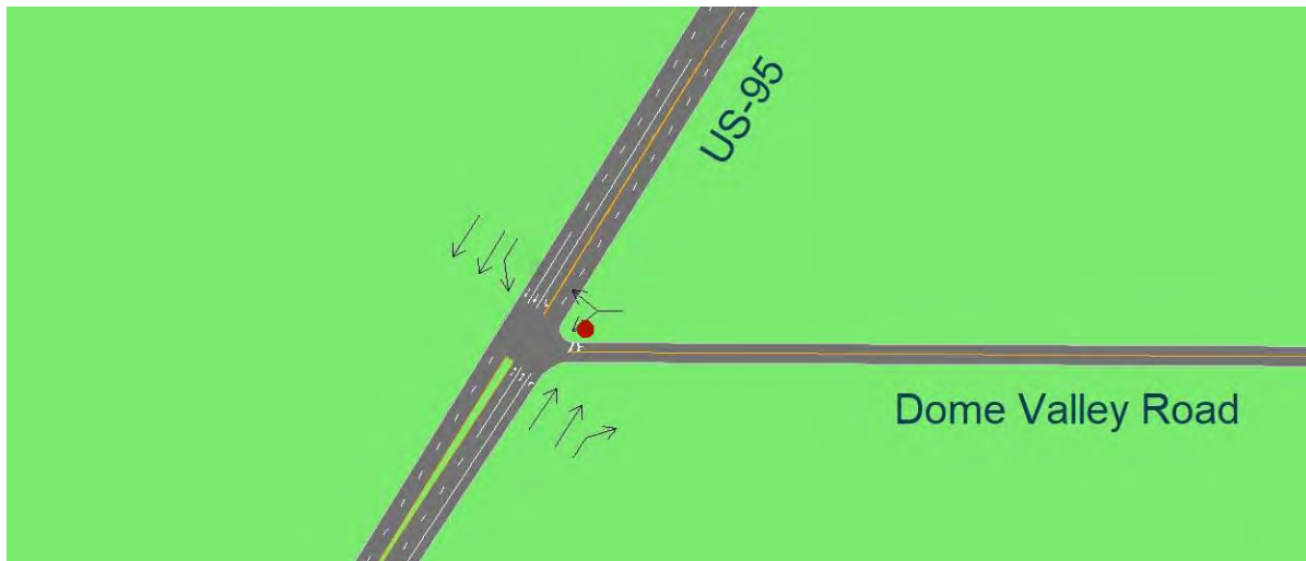
Figure 9 - Alternative 1 – Stop Controlled Intersection
