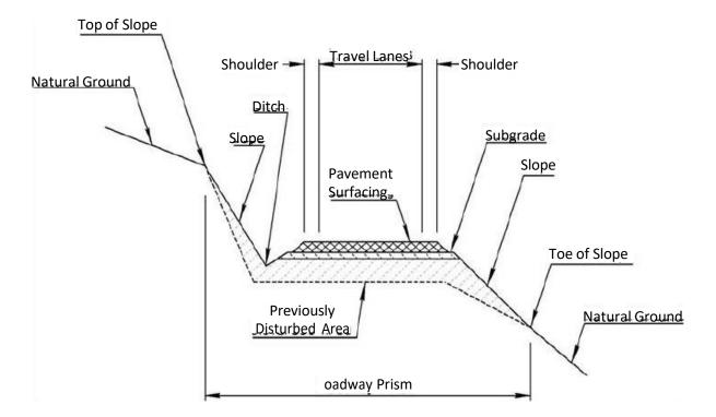
Figure 1. Illustration of Roadway Prism
