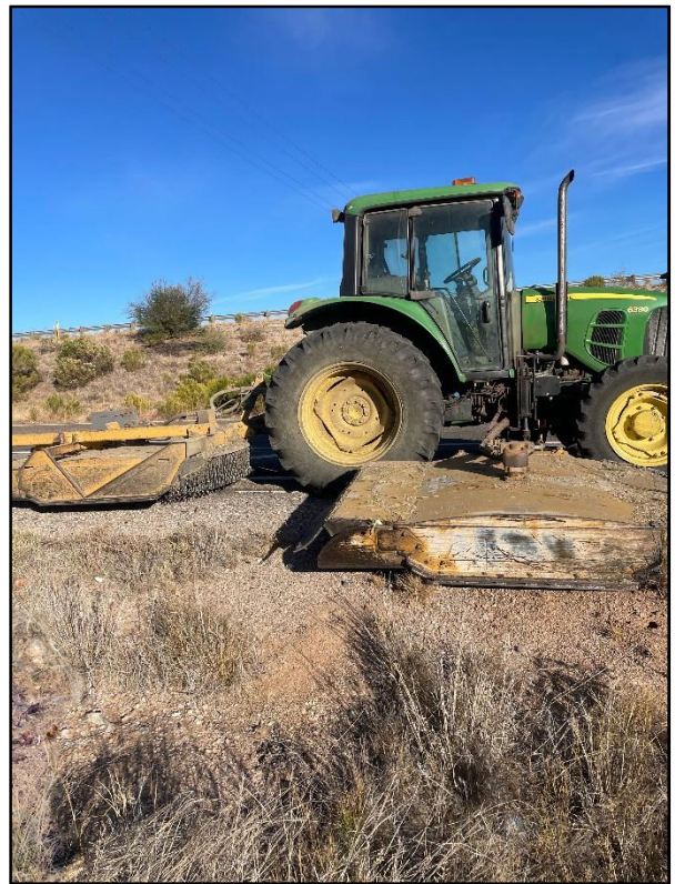
Two deck rotary mower can be used to mow one five foot swath or two swaths 10' wide total depending on the terrain.
