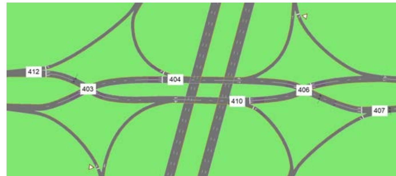
Figure 5.3 – DDI Intersection Diagram
