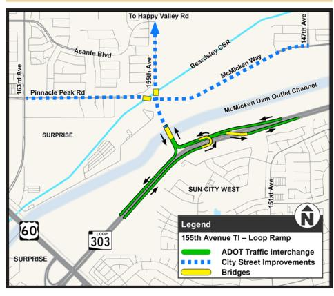
This alternative features a loop ramp configuration and braided ramps.
