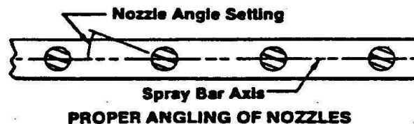
PROPER ANGLING OF NOZZLES
