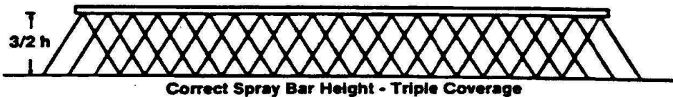
SPRAY BAR HEIGHT AND COVERAGE
