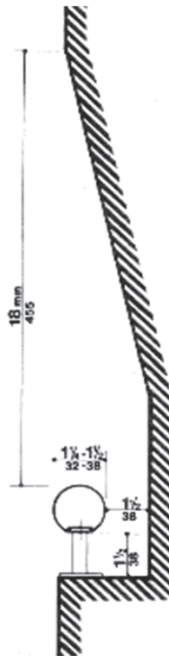
Figure 39d Size and Spacing of Handrails and Grab Bars Handrail
