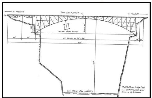
Hoffman dismissed the suspension design as too costly and, with a ten-ton load limit, too flimsy. Construction of a through arch, he maintained, would have necessitated the use of heavy overhead cableways to hoist the span halves into place. With the expense of returning the cables and tower materials prohibitively high, these would be abandoned at the site, adding considerably to the cost.
