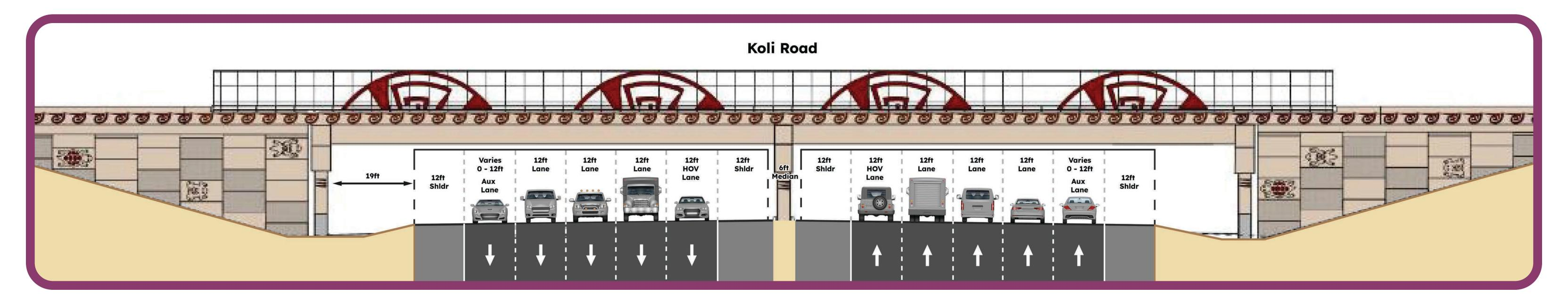
The proposed Koli Road Bridge would have two spans over I-10 and be constructed with precast, prestressed concrete girders.
