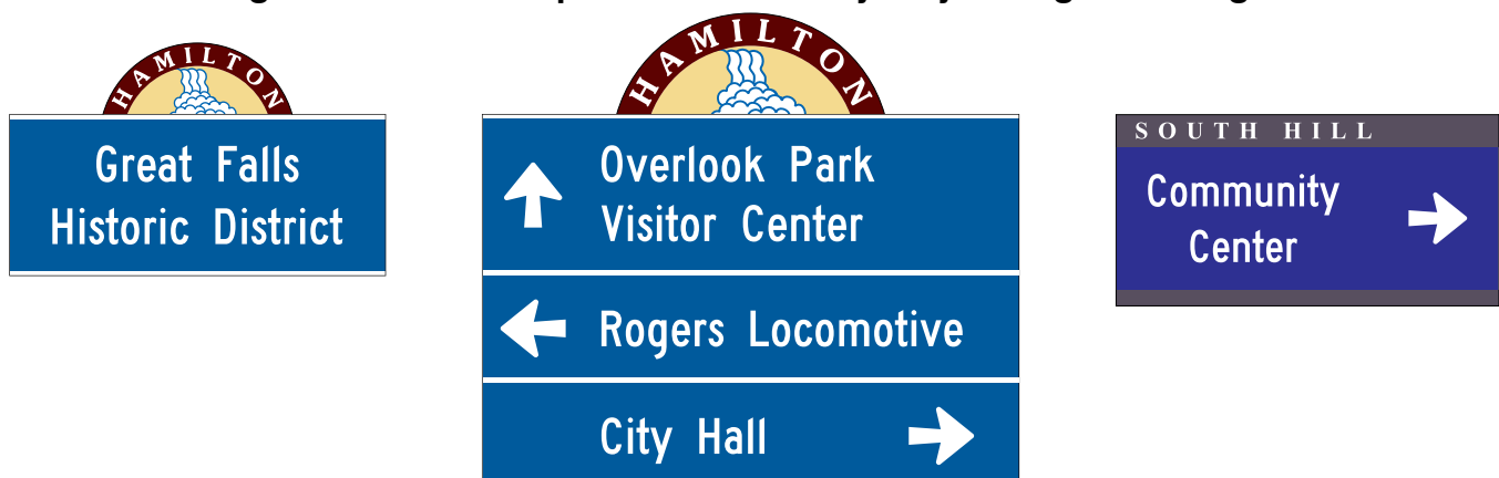
Figure 2D-30. Examples of Community Wayfinding Guide Signs
