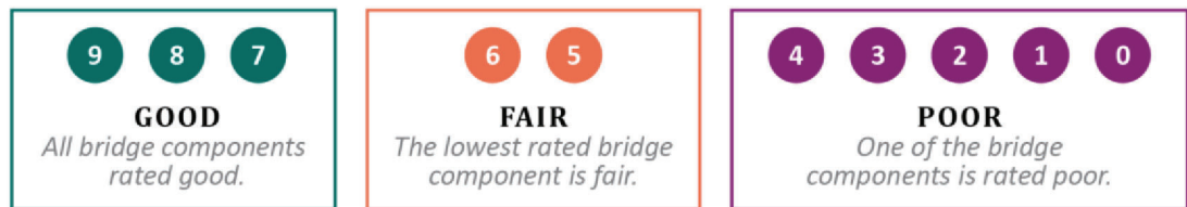
Figure 3-4 | National Bridge Inventory Bridge Rating Scale
