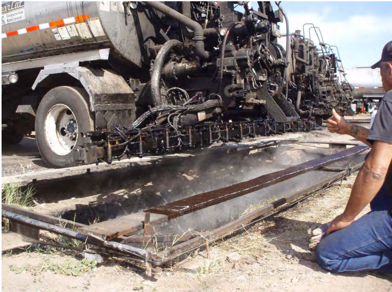
Typical "Sliding Platform" Testing Machine With Bituminous Material Being Sprayed
