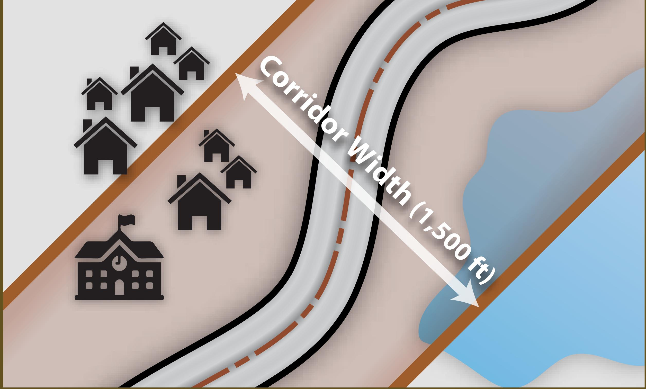
Evaluates design concepts for specific alignments within the corridor, such as 400 feet for a typical freeway alignment.
