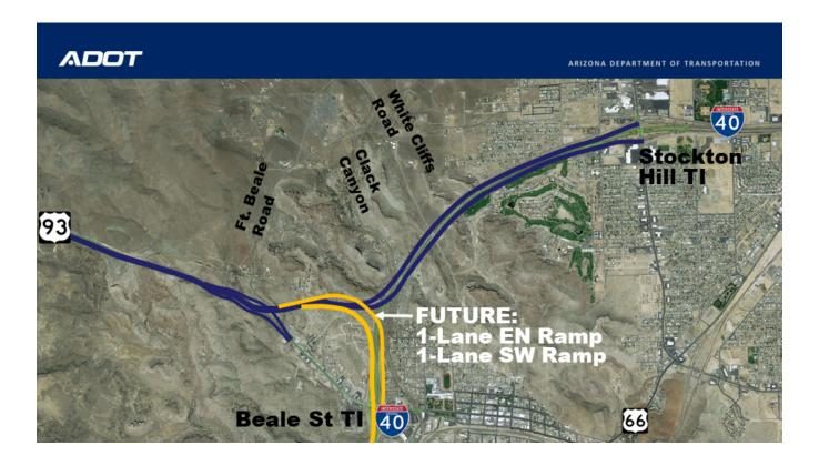
The final piece of the interchange improvement is the new ramps connecting US 93 to I-40 into California. These ramps will initially not carry much traffic, so they are not being constructed at first.
