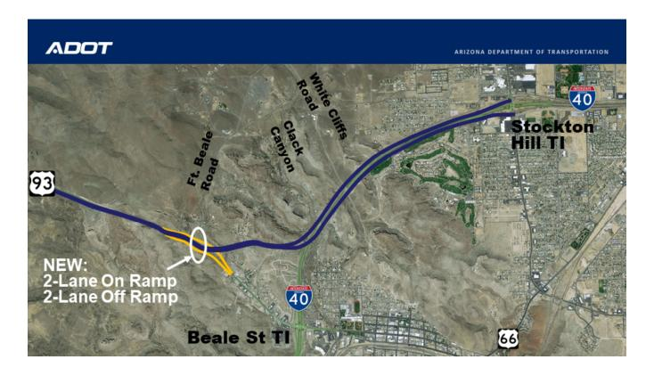
With the new connection now shown in blue, let's look at how we access Beale Street coming back from Vegas. Two new slip ramps will be constructed to maintain Eastbound and Westbound access directly for US 93 to Beale Street. During construction, it will be like spreading the existing road wider to fit the new freeway in the median. Westbound Beale will head around the north side of the improvement, with Eastbound Beale heading straight into town along the south side of the improvement.
