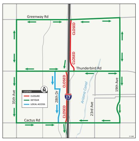
The closures are needed to install a new storm drain along the frontage road and connect it to the Arizona Canal Diversion Channel north of Dunlap Avenue.
