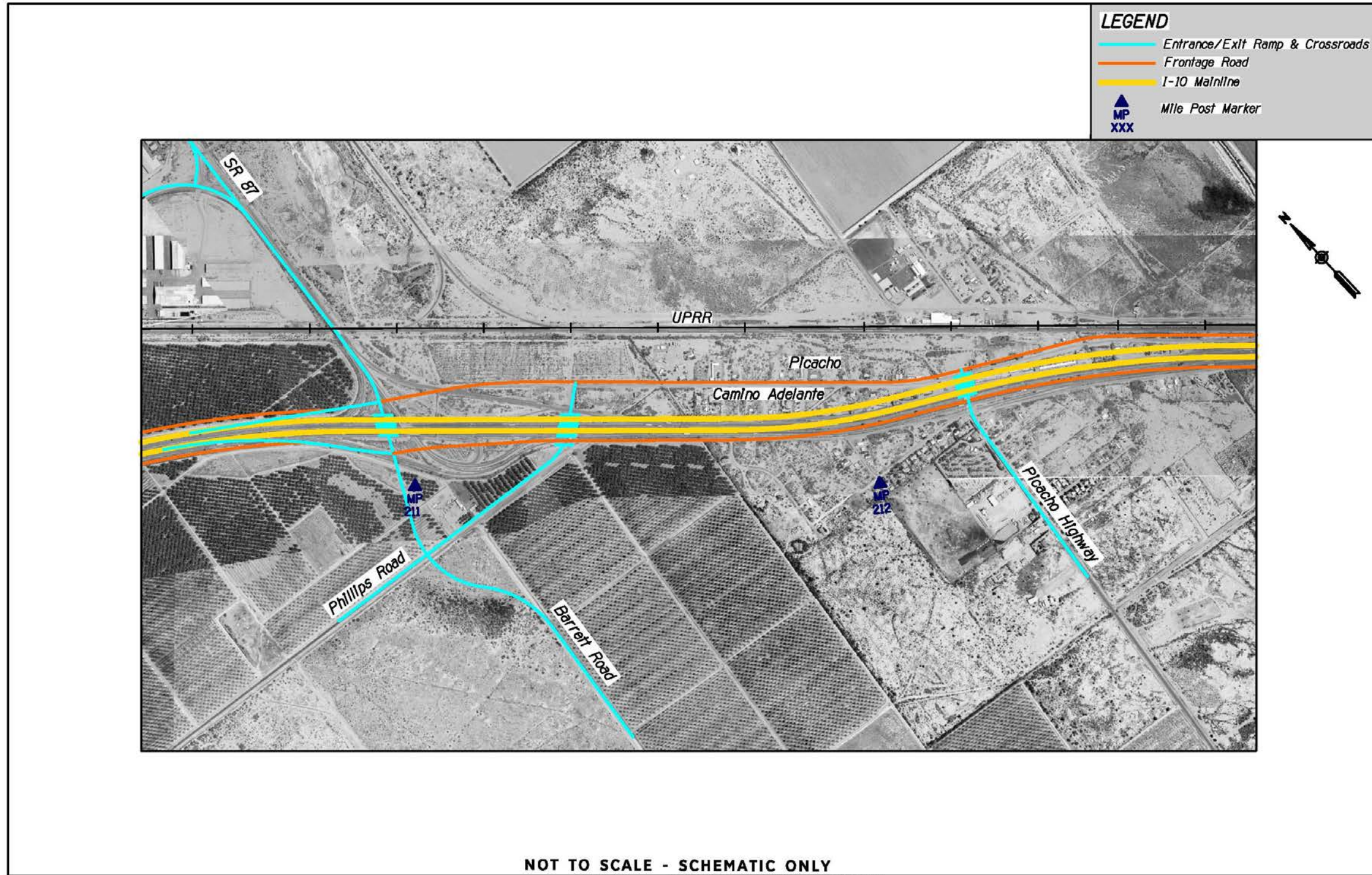
Figure 4.34 – SR 87 Interchange Alternative 1
