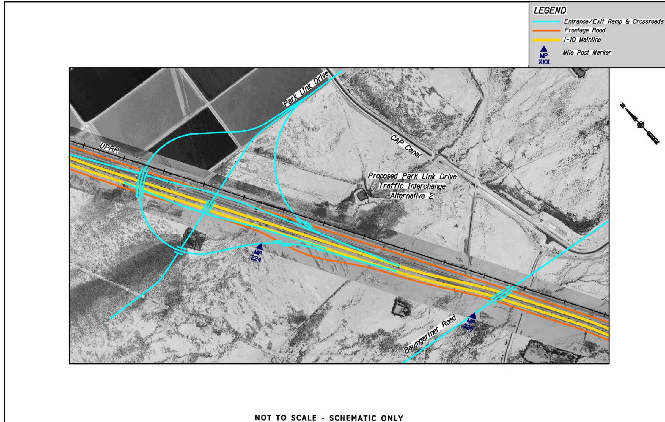
Figure 4.43 – Park Link Drive Interchange Alternative 2
