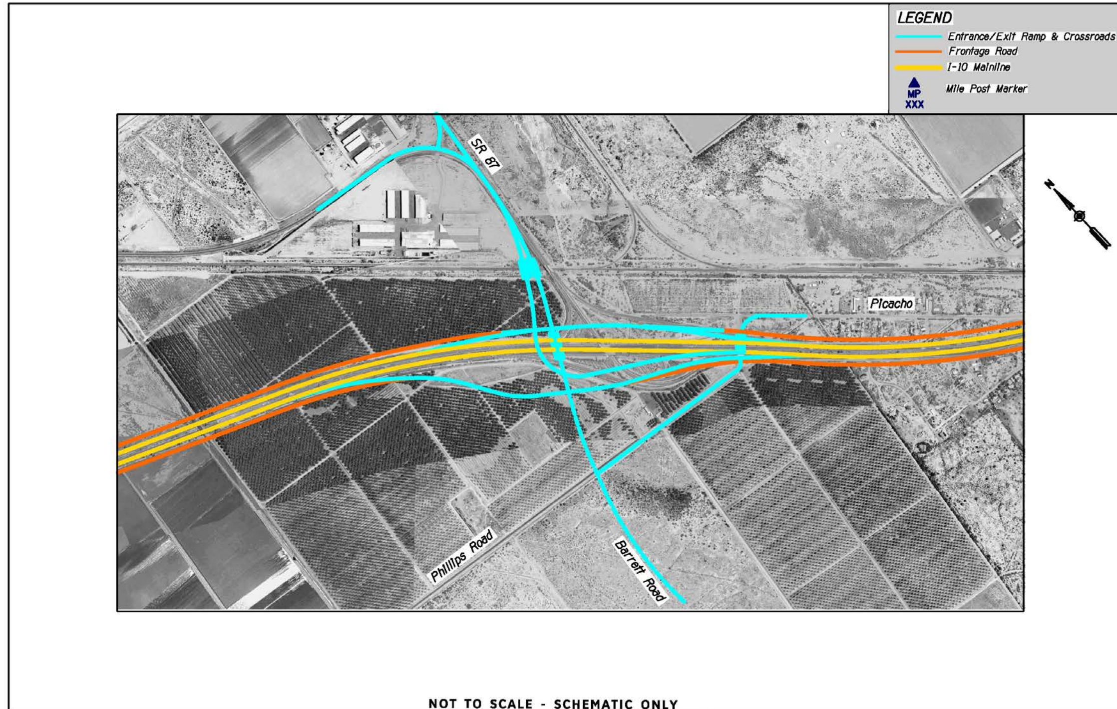
Figure 4.40 – SR 87 Interchange Alternative 7
